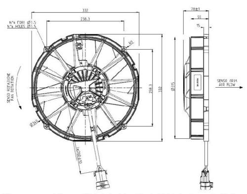
Fixing recommendation: use M6 bolts for fixing. Nominal tightening torque 3 +1/0 Nm Nominal torque defined for brand new, clean and lubricant-free bolts.
