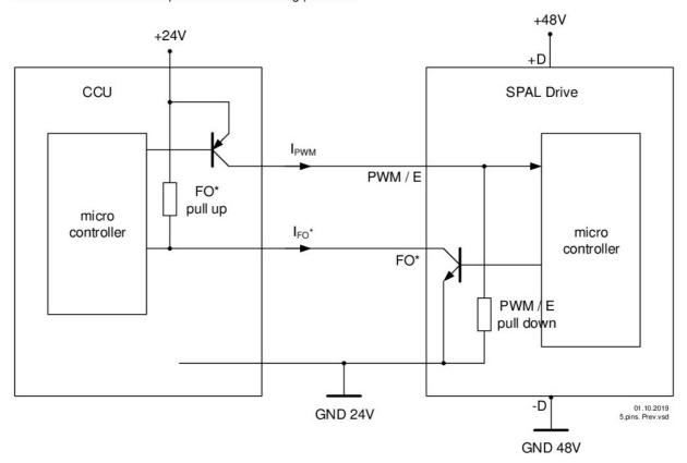
The CCU electronics and the Drive electronics are connected via two unidirectional lines.
