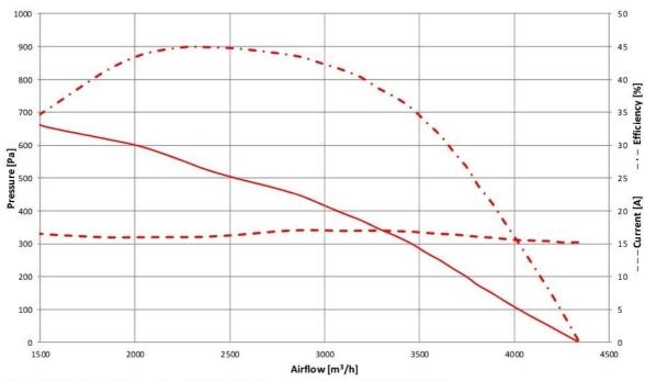
Air density 1.18 kg / m3 - Test number: #16082 – Test bench compliant to ANSI AMCA 210 TAMB = 20  $^{\circ}$ C ± 5  $^{\circ}$ C - UB = 48 V at the Drive connec tor
